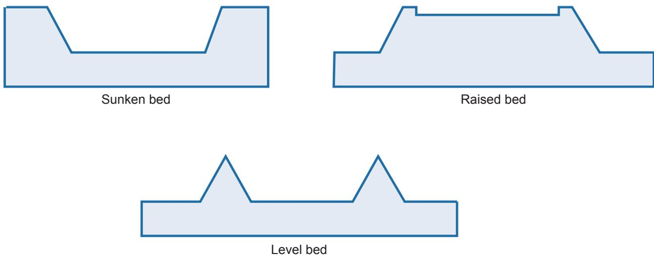
**Figure 3.2 Sunken, raised and level beds**
