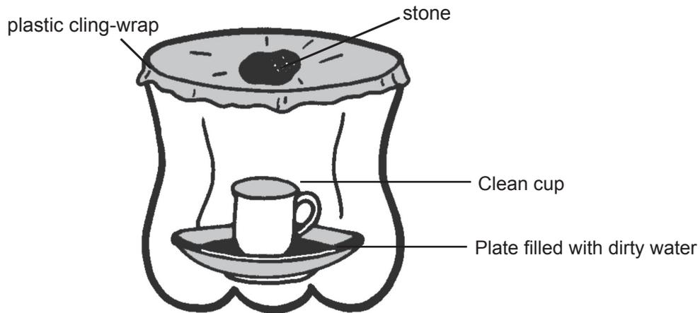
A. An evaporation/condensation chamber to simulate the water cycle.
